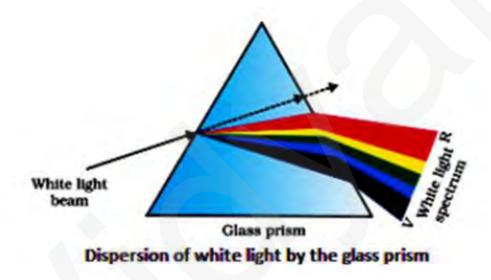
We see a beautiful band of seven colours on the screen called visible spectrum. The sequence of colours seen from the lower part of the screen is violet (V), indigo (I), blue (B), green (G), yellow (Y), orange (O) and red (R). The acronym for this is VIBGYOR
