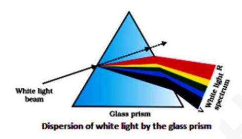
ii) Red light has the maximum wavelength and violet light has the minimum wavelength, so in a transparent medium except air and vacuum, red light having the largest wavelength suffers the least deviation while violet light having the least wavelength bends the most.
