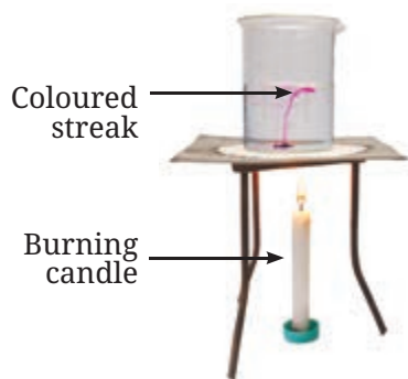
Fig. 7.5(b): Demonstration of convection in heated water
