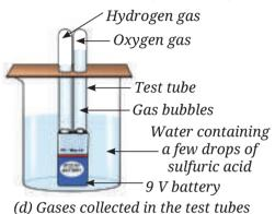
Fig. 8.8: Passing electricity through water
