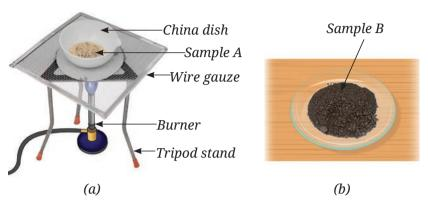
Fig. 8.15: (a) Heating Sample A; (b) Black mass
