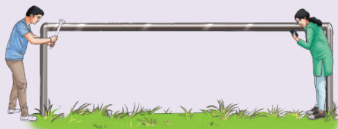
Fig. 10.23: Time difference between the sound reaching through air and steel
